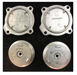
Intermediate Servo Cover. This will have a "C" cast on it. If your cover has an "A" or "B" letter on it then somebody has already swapped your tranny for a non-Hi-Po unit. The cover on the top left is from a 1966 transmission. The cover on the top right, with the heavier letter "C" is from a 1965 trans. The piston [bottom, left]) of the 1966 servo cover has a Ford oval logo. The 1965 piston [bottom, right] is a re-pop (there is no Ford logo).
