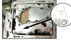
The Valve Body in the Hi-Po C4 is special, and has settings calibrated for the 289 Hi-Po engine. The stock Hi-Po valve body will have a "1U" tag on it. Make sure they save this tag.
