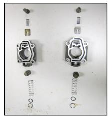
The other part unique to the Hi-Po C4 is the Governor Assembly. It has a lightened secondary counterweight that allows the trans to shift at a higher rpm in "drive" than the standard model C4. A standard C4 shifts at WOT (wide open throttle) at around 4500-5000 rpm. The Hi-Po C4 shifts at WOT at around 5000-6000 rpm. The factory Hi-Po governor has a white paint stripe on it. Stock governor is pictured on the right; Hi-Po governor is on the left.
