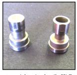
Secondary Counterweights in detail. Hi-Po counterweight on the right has been machined to reduce weight. This results in higher rpm shifts.
